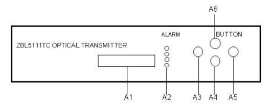
A1: LED display window, which can display the output laser power P(mw), the laser bias current BI(mA), temperature  $T(^{\circ}C)$ , cooling current RC(A), and electric power detection of +24.4V,+5.4V,-5.45V and IP address, gateway, OMI value, the temperature in the machine and so on.
